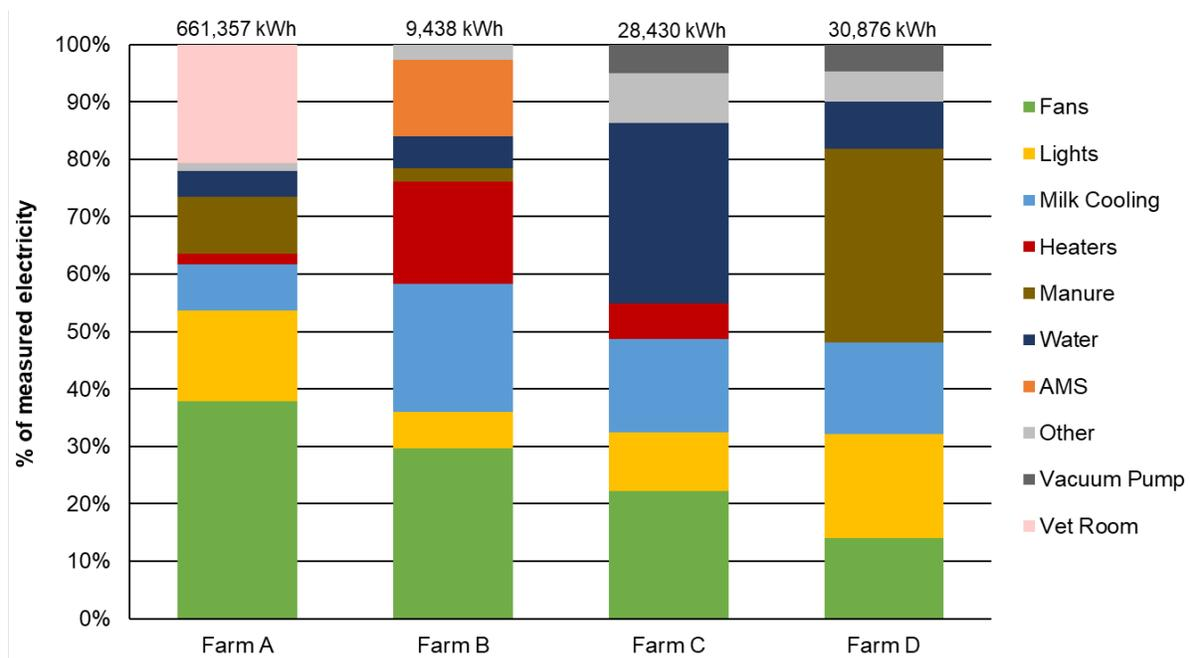
The average monthly electricity use measured by data loggers and the percent used by each electrical load category. The average monthly total electricity in kWh is displayed at the top of each bar.
