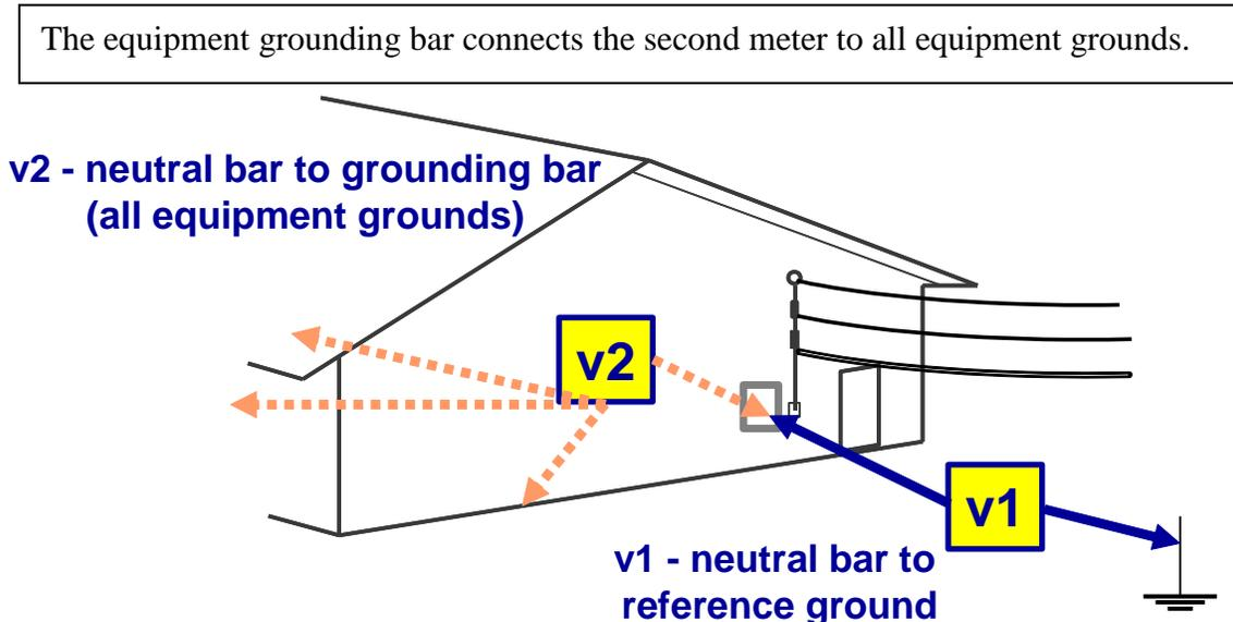
**\*\***Removing the neutral conductors versus the equipment grounding conductors may be more practical because the neutral conductors are insulated therefore easier to keep from touching each other while doing this test.
