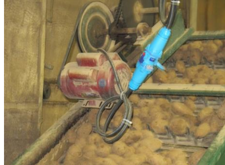
TYPICAL ELEVATOR MOVED INTO PLACE AND FIELD CONNECTED
