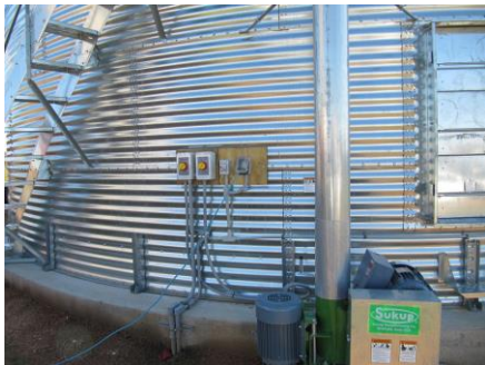
EACH BIN HAS MANY FAN MOTORS ALONG WITH THE LP GAS FIRED UNITS
