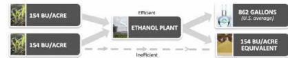
Fig. 4 Returning one bushel of corn for every two used. Nearly all corn consumed by ethanol plants comes from the feed corn supply, but since corn ethanol returns livestock feed to the market, the net corn disappearance due to ethanol is only one-half the gross corn consumption of the plant. According to Dr. Terry Klugebein of the University of Nebraska, on a dry weight basis, 33% of the corn is left for utilization as livestock feed in the form of distiller grain. But since DDG has 145% the feed value of raw corn, the net effect is that for every two bushels of corn used to make ethanol, one bushel of feed equivalent is returned. Source: Ethanol Access America
