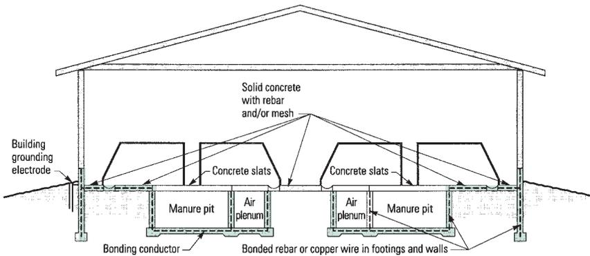
**Equipotential Plane in a Building with Fully Slatted Floors**
