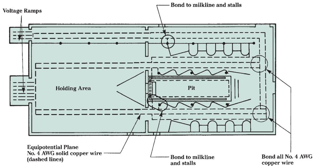
Figure 4. Equipotential Plane in a Milking Parlor/Holding Area
