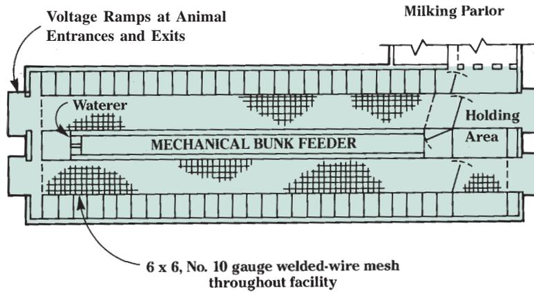
Figure 6. Transition Area/Voltage Ramp
