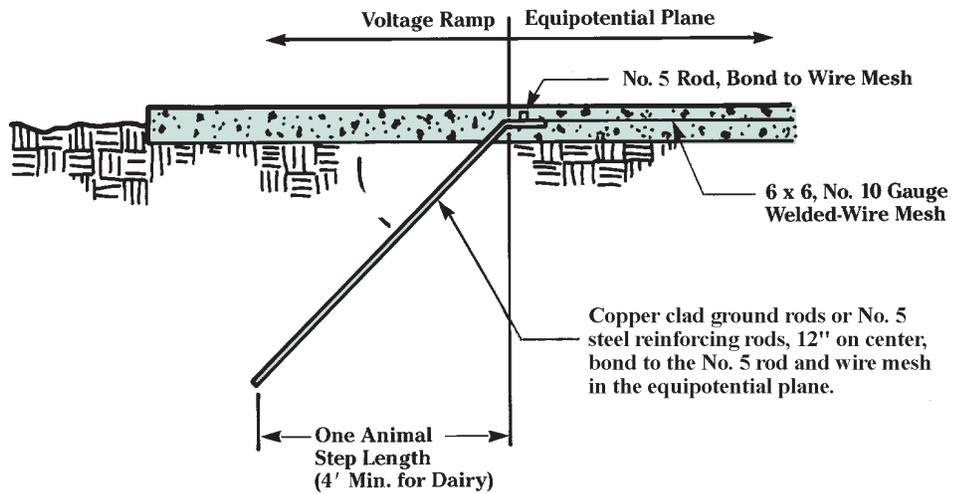
Figure 7. Equipotential Plane in a Stanchion/Tie-Stall Barn
