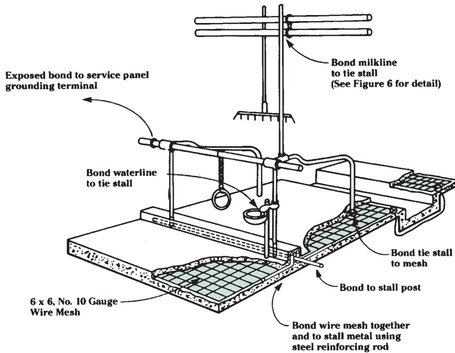
Figure 8. Retrofit Equipotential Plane in a Stanchion/Tie-Stall Barn
