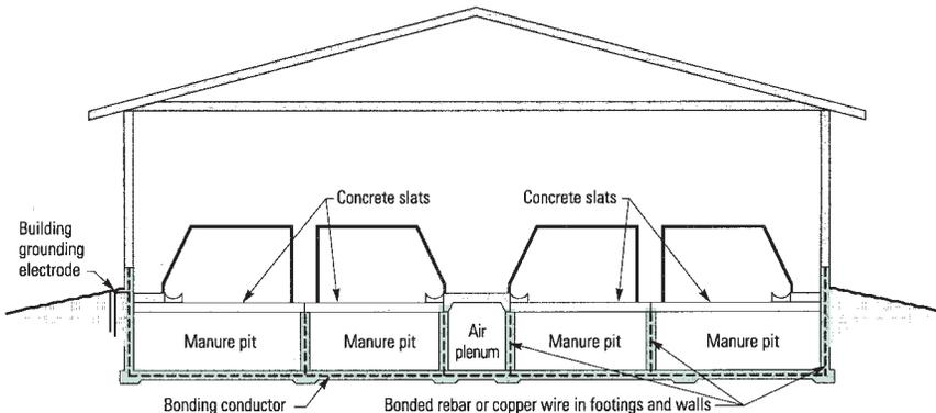
**Figure 10. Equipotential Plane in a Water and Bunk Feeder Area**
