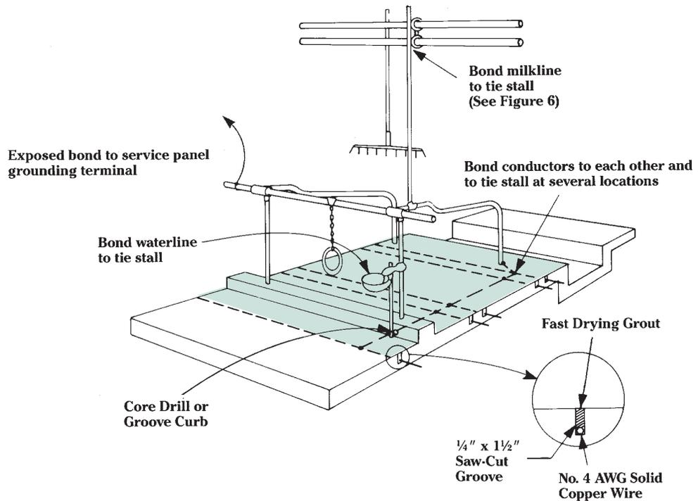
**Figure 9. Equipotential Plane in a Building with Partly Slatted Floors**
